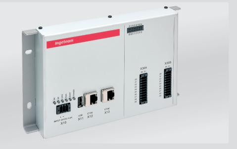
INGESYS<sup>™</sup> CMS is a customizable and internally modular online monitoring system, that anticipates the appearance of functional anomalies in the machine, based on the analysis of its variables (vibrations, temperature, position, etc.).
